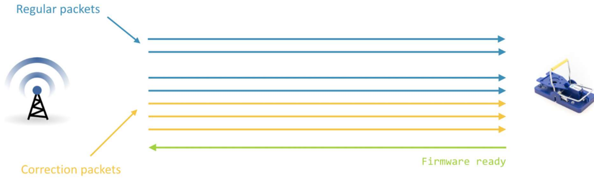
Figure 3: The network delivers the regular packets first, then sends correction packets. Devices that have missed packets can recover these packets through the generic correction packets, rather than request a re-transmission.
