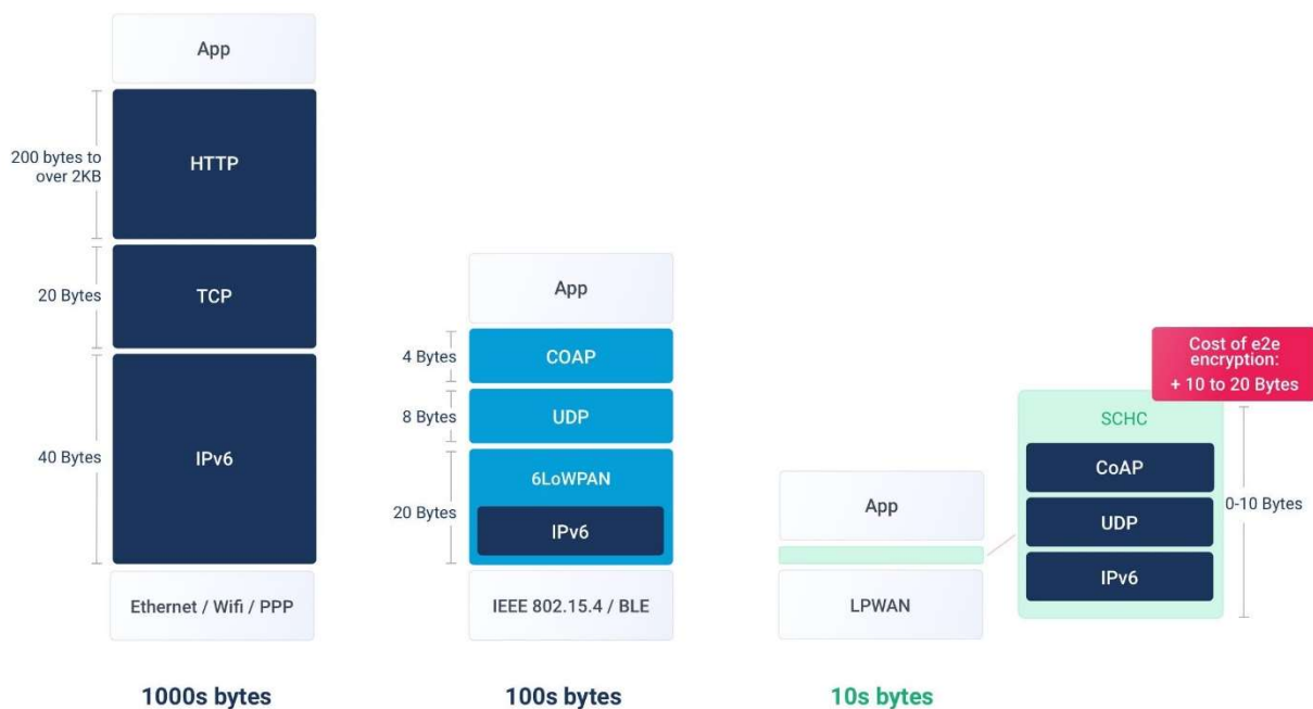
Figure 4: Internet Protocol stack compared to 6LoWPan and SCHC compression frameworks on IPv6/UDP/CoAP
