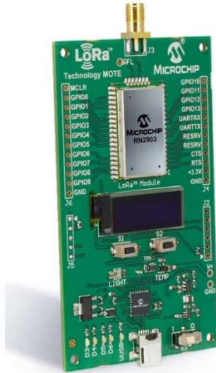
Figure 3: Microchip DM164139 LoRa Mote Board is certified via the LoRa Alliance comprehensive certification program
